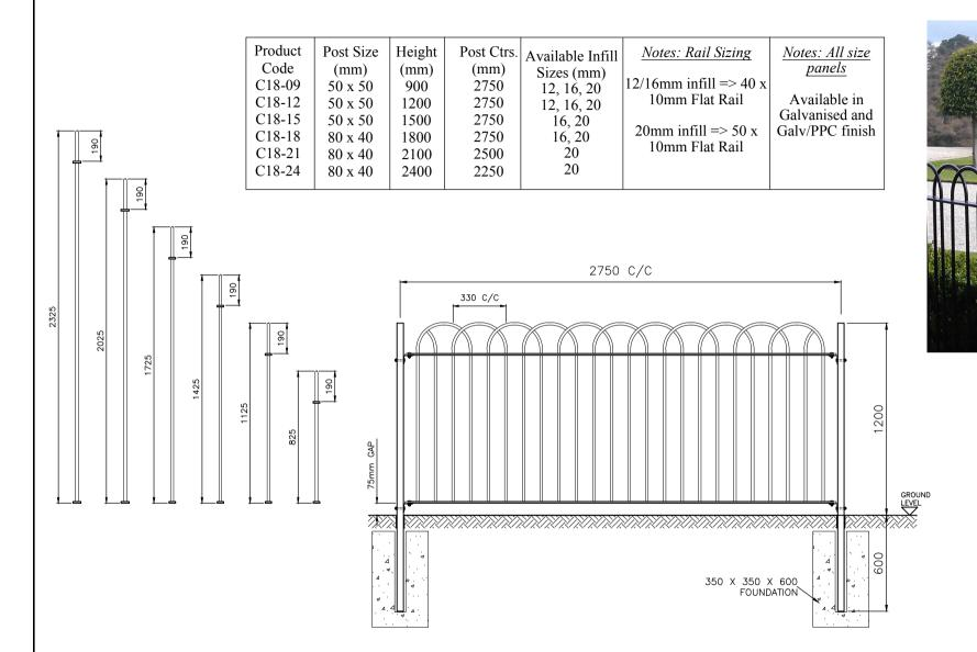
Please Note: Post Centre illustrated is based on a railing of 1200mm high using a Ø16mm infill.
