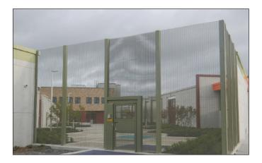
A very high level of security is afforded by Kilmainham 358 mesh. Kilmainham panels are constructed using 4mm vertical and horizontal wires, the aperture of the mesh is 12.5mm x 75mm (in old imperial measurement system this equated to 3 inches x .5 inch x 8g i.e. 358).
